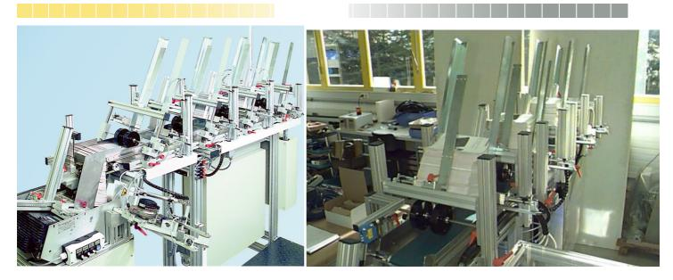
For a customer we manufactured a feeder that is assembled with a multiple magazine where the shafts are built up consecutively.
