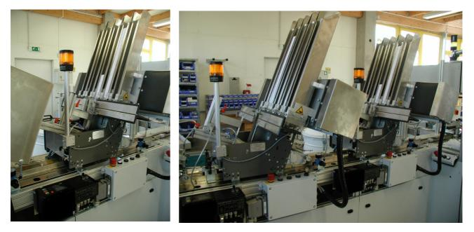
Multipe magazine for small products (phone cards) to increase feeders' autonomy. The magazine is equipped with 5 shafts that are emptied automatically one after the next and convey the products to the feeder. The shafts are exchangeable so that they can be refilled "externally" without stopping the machine.
